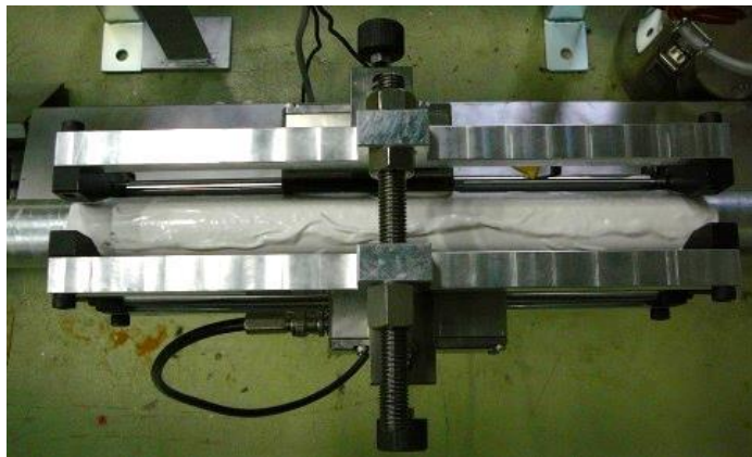
Fig. 18 25A(1 inch) Steam Pipe Setup.
